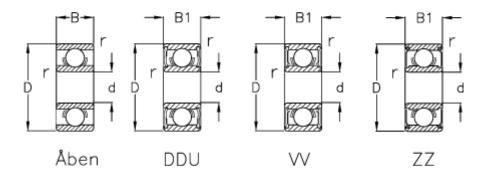
Max rpm ZZ-WW = 36000 В = 6 В1 = 6 r min = 0.3Type d = 8 =698D = 19 Load Cor (N) = 910Load Cr (N) = 2240 Max rpm DD = 28000Max rpm open = 43000
